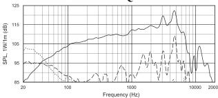
Distortion measurements taken with an input of 15.5V @ 1 meter (30 watts at 8 ohms). Distortion levels shown have been raised by 20 dB. The dashed line shows 2nd harmonic and the dotted line shows the 3rd harmonic. Note lack of 3rd harmonic at high frequencies.
